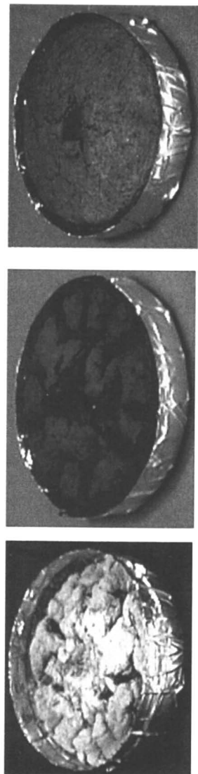
Figure 9. Digitized photos of gasification residues from PP/5 % MMT (SCPX1980) (left), PP/15 % PPgMA/2 % MMT (SCPX1980) (center), and PP/15 % PPgMA/5 % MMT (SCPX1980) (right).
